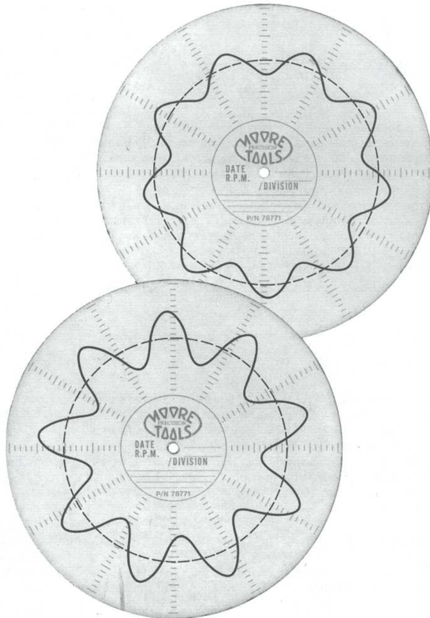
FIGURE CD14.1 Spherical roller bearing inner ring waviness, machine setup error. Each radial division equals 1\ \mu\text{m} .
